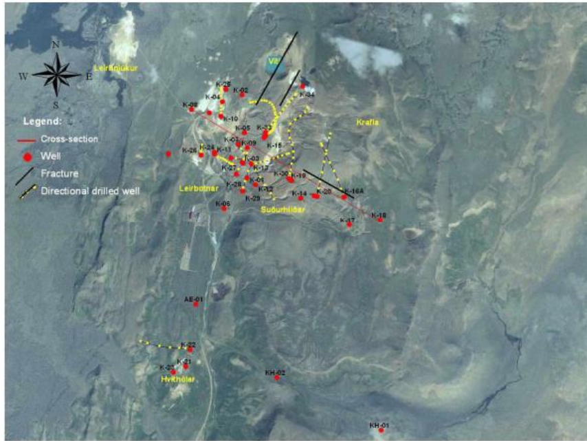
Figure 6: Location map of drill holes at Krafla. Trajectories for inclined wells are indicated. The cross-section location from well KJ-8 across the field to KJ-18 is shown. More information is in [9].
