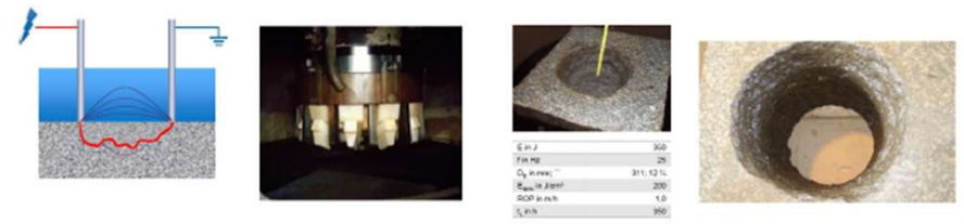
Figure 1 EPP rock breaking principle
