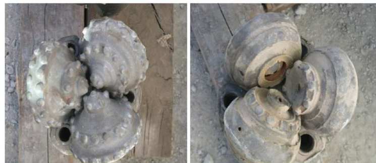
Image of drill-bit tear from the Geysers EGS Demonstration Project
