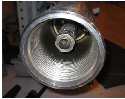
Figure 14: Male extender installed in collar
