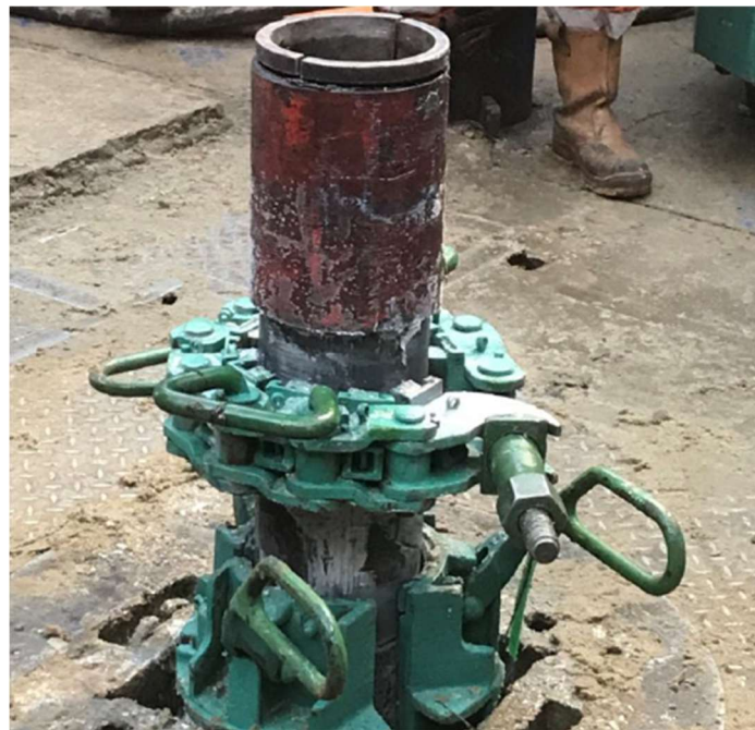
Figure 24. Drill collar in rotary table slips with safety collar on top.
