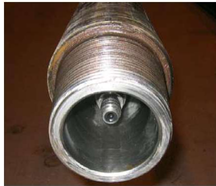
Figure 15: Female extender installed in collar
