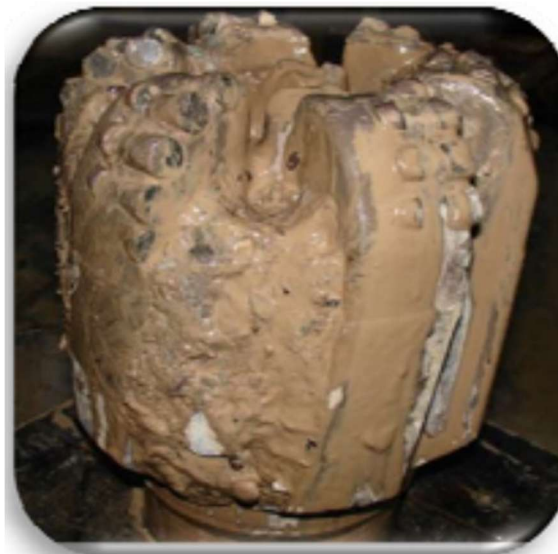
Figure 3. Balled up PDC bit. Bit balling can occur in water sensitive formations and mainly happens with water-based muds. Therefore, the EPP tools will need to have a proper JSA and several adjustable nozzles to optimize bit cleaning.
