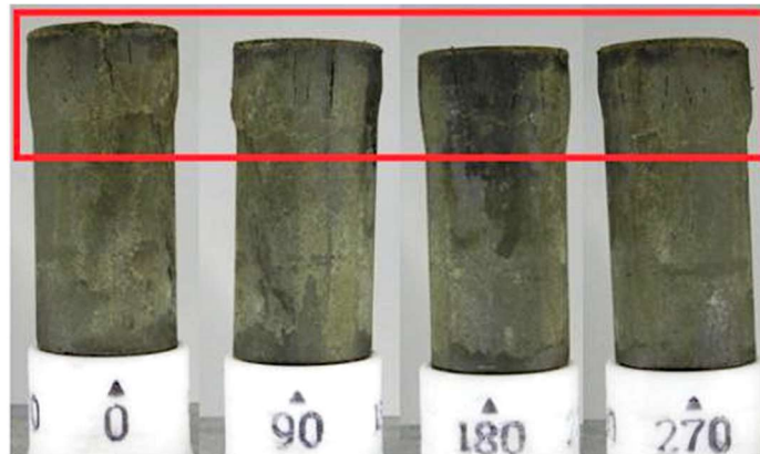
Figure 2. (unpublished work by Mileva Radonjic Research Group) shows OPC-based blended cement with Graphene Nanoplatelets (GNP) stored for 9 months in the Newberry geothermal well, demonstrating resistance to brittle fracturing after UCS testing.
