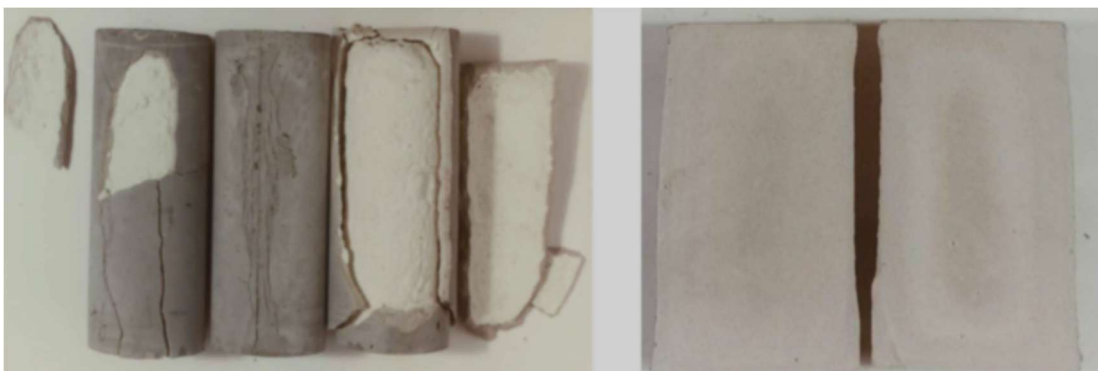
Figure 1. The impact of carbonation on the degradation of OPC cores. On the left, the figure shows neat OPC cement cores. On the right are sliced OPC cores with added silica flour. Both cores were subjected to 260^\circ\text{C} for 4 months. Source: Milestone et al.
